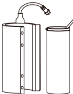
MP270P-BD20 Compatible Diameter: 7-8cm Max. Printable Length: 20.3cm
