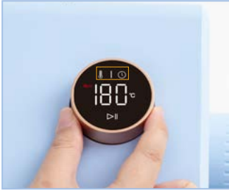
3 Tap and rotate the knob to set time and temperature.
