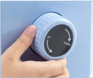
5 Turn the pressure knob to apply appropriate pressure to the mug.
