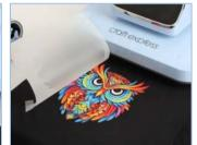
4 Push the lower platen back, and the heat press will start printing automatically. Once the printing is complete, remove the printed items. Repeat the process to print your items in batches.
