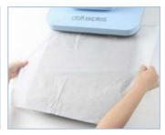
2 Pull out the drawer and place a sheet of protective paper on the mat.
