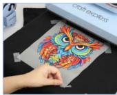
3 Place the t-shirt on the mat and fix the image onto the t-shirt with heat resistant tap.
